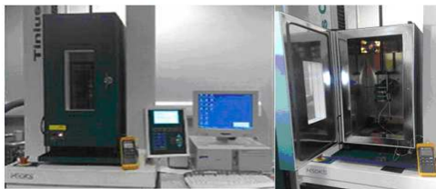
Figure (1):- (a) Environmental Chamber Shown Mounted on Frame and between Columns of Tinius Olsen Test Machine (b) Foam Testing
