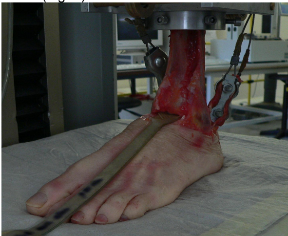
Figure 1: Experimental set-up with the cadaver foot in the Zwick machine with the AJP sensor placed inside the tibiotalar joint.
